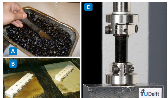
Mortar testing: Material Response parameters, obtained from Dynamic Mechanical Analysis [C] on mortar [A] samples [B], were used as an input for the Finite Element Model.
