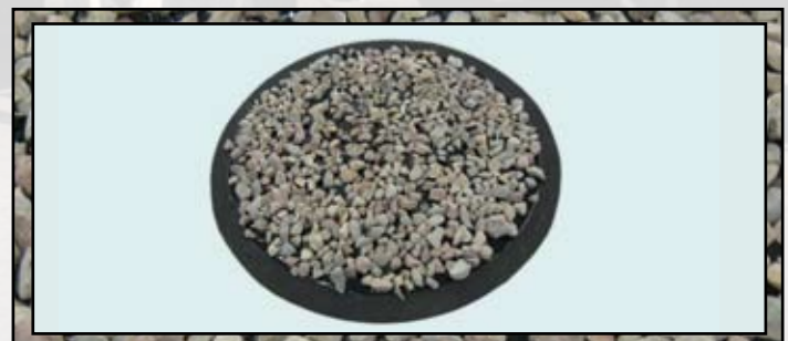
Figure 2 - Kraton D1192-Modified CRS-2P Emulsion Sweep Test Pad - Post-Sweep
